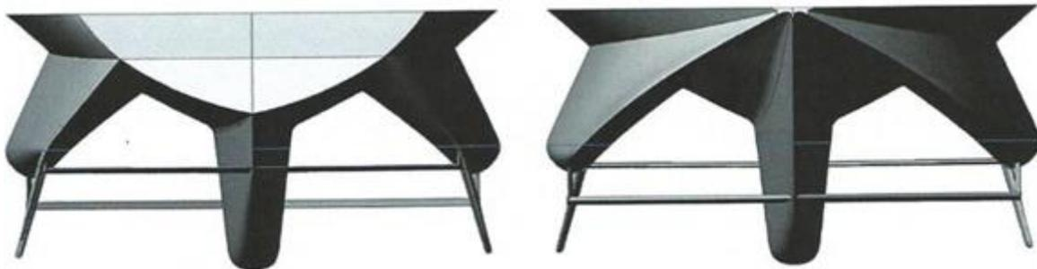
Figure 3: **Before and after of Optimisation using CFD** Credits: [AnwigemA B.V](#)
